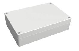
Hammond enclosure, NEMA 4/4X/6/6P/12/13, 180 x 120 x 46mm (HxWxD), polycarbonate, RAL 7035 light gray, screw cover, purchase subpanel separately.
