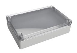
Hammond enclosure, NEMA 4/4X/6/6P/12/13, 180 x 120 x 46mm (HxWxD), polycarbonate, RAL 7035 light gray, clear polycarbonate screw cover, purchase subpanel separately.
