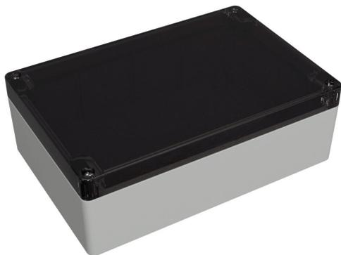
Hammond enclosure, NEMA 4/4X/6/6P/12/13, 180 x 120 x 61mm (HxWxD), polycarbonate, RAL 7035 light gray, smoke polycarbonate screw cover, purchase subpanel separately.
