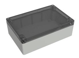
Hammond enclosure, NEMA 4/4X/6/6P/12/13, 180 x 120 x 61mm (HxWxD), polycarbonate, RAL 7035 light gray, clear polycarbonate screw cover, purchase subpanel separately.
