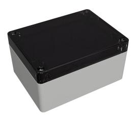
Hammond enclosure, NEMA 4/4X/6/6P/12/13, 120 x 90 x 61mm (HxWxD), polycarbonate, RAL 7035 light gray, smoke polycarbonate screw cover, purchase subpanel separately.
