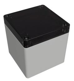
Hammond enclosure, NEMA 4/4X/6/6P/12/13, 90 x 90 x 91mm (HxWxD), polycarbonate, RAL 7035 light gray, smoke polycarbonate screw cover, purchase subpanel separately.
