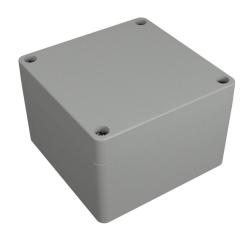
Hammond enclosure, NEMA 4/4X/6/6P/12/13, 90 x 90 x 61mm (HxWxD), polycarbonate, RAL 7035 light gray, screw cover, purchase subpanel separately.
