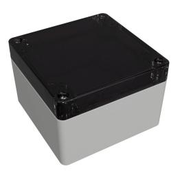
Hammond enclosure, NEMA 4/4X/6/6P/12/13, 90 x 90 x 61mm (HxWxD), polycarbonate, RAL 7035 light gray, smoke polycarbonate screw cover, purchase subpanel separately.
