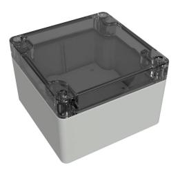
Hammond enclosure, NEMA 4/4X/6/6P/12/13, 90 x 90 x 61mm (HxWxD), polycarbonate, RAL 7035 light gray, clear polycarbonate screw cover, purchase subpanel separately.
