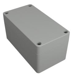
Hammond enclosure, NEMA 4/4X/6/6P/12/13, 120 x 65 x 61mm (HxWxD), polycarbonate, RAL 7035 light gray, screw cover, purchase subpanel separately.
