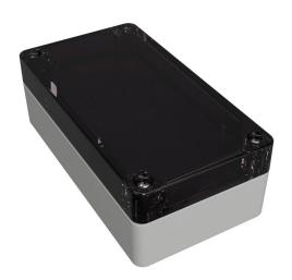
Hammond enclosure, NEMA 4/4X/6/6P/12/13, 120 x 65 x 41mm (HxWxD), polycarbonate, RAL 7035 light gray, smoke polycarbonate screw cover, purchase subpanel separately.
