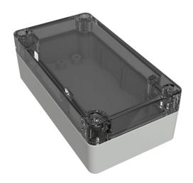
Hammond enclosure, NEMA 4/4X/6/6P/12/13,  $120 \times 65 \times 41$ mm (HxWxD), polycarbonate, RAL 7035 light gray, clear polycarbonate screw cover, purchase subpanel separately.
