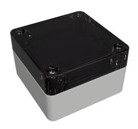
Hammond enclosure, NEMA 4/4X/6/6P/12/13, 65 x 65 x 41mm (HxWxD), polycarbonate, RAL 7035 light gray, smoke polycarbonate screw cover, purchase subpanel separately.
