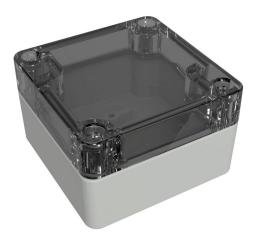
Hammond enclosure, NEMA 4/4X/6/6P/12/13, 65 x 65 x 41mm (HxWxD), polycarbonate, RAL 7035 light gray, clear polycarbonate screw cover, purchase subpanel separately.
