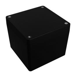
Hammond enclosure, NEMA 1/4/4X/12/13, 121 x 121 x 102mm (HxWxD), die-cast aluminum alloy, black, powder coat finish, screw cover.
