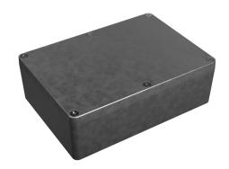
Hammond enclosure, NEMA 1/4/4X/12/13, 171 x 121 x 55mm (HxWxD), die-cast aluminum alloy, screw cover.
