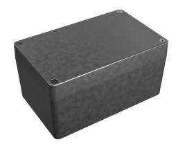
Hammond enclosure, NEMA 1/4/4X/12/13,  $160 \times 100 \times 81$ mm (HxWxD), die-cast aluminum alloy, screw cover.
