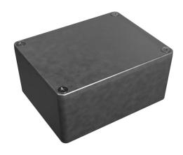
Hammond enclosure, NEMA 1/4/4X/12/13,  $115 \times 90 \times 55$ mm (HxWxD), die-cast aluminum alloy, screw cover.
