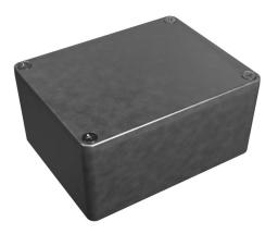
Hammond enclosure, NEMA 1/4/4X/12/13, 115 x 90 x 55mm (HxWxD), die-cast aluminum alloy, screw cover.
