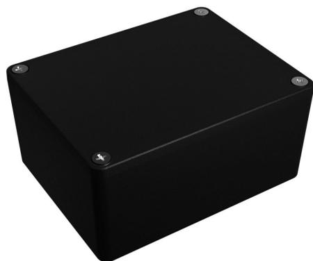
Hammond enclosure, NEMA 1/4/4X/12/13, 115 x 90 x 55mm (HxWxD), die-cast aluminum alloy, black, powder coat finish, screw cover.
