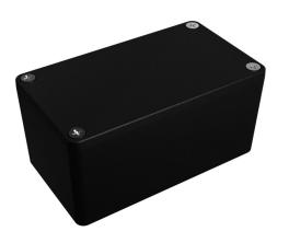
Hammond enclosure, NEMA 1/4/4X/12/13, 115 x 65 x 55mm (HxWxD), die-cast aluminum alloy, black, powder coat finish, screw cover.
