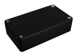
Hammond enclosure, NEMA 1/4/4X/12/13, 115 x 65 x 30mm (HxWxD), die-cast aluminum alloy, black, powder coat finish, screw cover.
