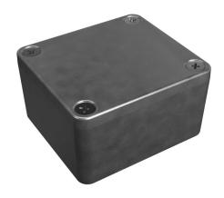
Hammond enclosure, NEMA 1/4/4X/12/13, 64 x 58 x 35mm (HxWxD), die-cast aluminum alloy, screw cover.
