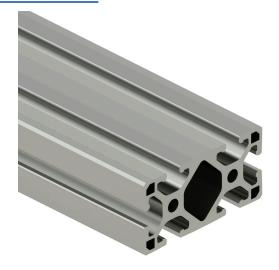
SureFrame 15 Series light T-slotted rail, silver, 6063-T6 anodized aluminum alloy, cut to length, 1.5 x 3in profile, slot size 8.
