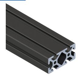
SureFrame 15 Series standard T-slotted rail, black, 6063-T6 anodized aluminum alloy, cut to length, 1.5 x 3in profile, slot size 8.
