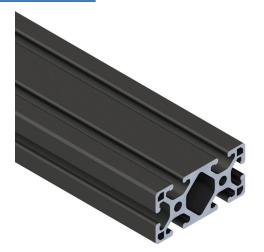
SureFrame 15 Series light T-slotted rail, black, 6063-T6 anodized aluminum alloy, cut to length, 1.5 x 3in profile, slot size 8.
