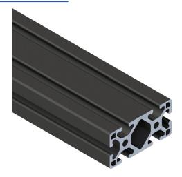
SureFrame 15 Series light T-slotted rail, black, 6063-T6 anodized aluminum alloy, cut to length, 1.5 x 3in profile, slot size 8.
