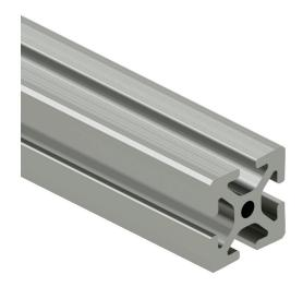
SureFrame 15 Series standard T-slotted rail, silver, 6063-T6 anodized aluminum alloy, cut to length,  $1.5 \times 1.5$ in profile, slot size 8.
