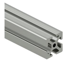
SureFrame 15 Series standard T-slotted rail, silver, 6063-T6 anodized aluminum alloy, cut to length,  $1.5 \times 1.5$  in profile, slot size 8.
