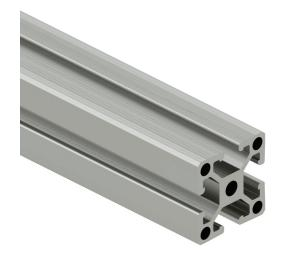
SureFrame 15 Series ultra light T-slotted rail, silver, 6063-T6 anodized aluminum alloy, cut to length, 1.5 x 1.5in profile, slot size 8.
