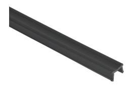
FATH cover profile, black, 2000mm, polypropylene, slot size 10. Package of 25. For use with all 45mm and 90mm profile T-slotted rails. Manufacturer part number: 092041.
