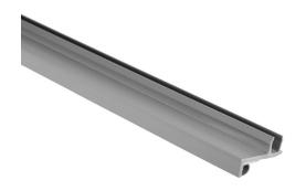
FATH sealing strip, gray, 2000mm, PVC/TPE, slot size 10. Package of 2. For use with all 45mm and 90mm profile T-slotted rails. Manufacturer part number: 092259.
