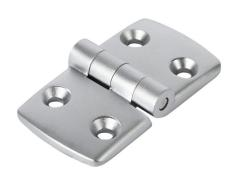
FATH non-detachable combination hinge, silver, die-cast aluminum, slot size 10. For use with all 45mm and 90mm profile T-slotted rails. Manufacturer part number: 095A4545FS20.
