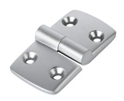
FATH right-hand detachable combination hinge, silver, die-cast aluminum, slot size 10. For use with all 45mm and 90mm profile T-slotted rails. Manufacturer part number: 095A4545RS20.
