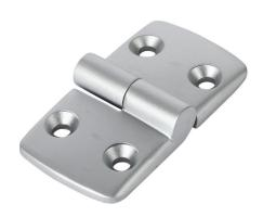
FATH left-hand detachable combination hinge, silver, die-cast aluminum, slot size 10. For use with all 45mm and 90mm profile T-slotted rails. Manufacturer part number: 095A4545LS20.
