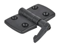
FATH non-detachable combination hinge with locking lever, black, fiberglass reinforced plastic, slot size 10. For use with all 45mm and 90mm profile T-slotted rails. Manufacturer part number: 095KF4545F10.
