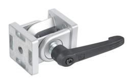
FATH pivot joint with locking handle, silver, 178-degree adjustable, 2 holes, die-cast zinc, slot size 10. For use with all 45mm and 90mm profile T-slotted rails. Manufacturer part number: 093GF45AN.
