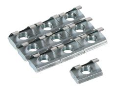
FATH roll-in nut, silver, M8-1.25, zinc plated steel, slot size 10. Package of 10. For use with all 45mm and 90mm profile T-slotted rails. Manufacturer part number: 096168F.
