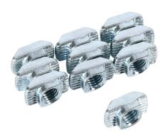
FATH hammer nut, silver, M8-1.25, zinc plated steel, slot size 10. Package of 10. For use with all 45mm and 90mm profile T-slotted rails. Manufacturer part number: 096H10830.
