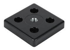
FATH transport/base plate, black, 80 x 80mm, M12-1.75, die-cast zinc. For use with 80 x 80mm profile T-slotted rails. Mounting hardware included. Manufacturer part number: 093T80801208S.
