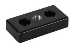
FATH transport/base plate, black, 40 x 80mm, M12-1.75, die-cast zinc. For use with 40 x 80mm profile T-slotted rails. Mounting hardware included. Manufacturer part number: 093T40801208S.
