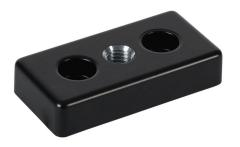
FATH transport/base plate, black, 40 x 80mm, M12-1.75, die-cast zinc. For use with 40 x 80mm profile T-slotted rails. Mounting hardware included. Manufacturer part number: 093T40801208S.
