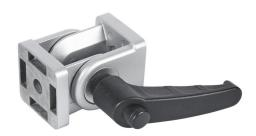
FATH pivot joint with locking handle, silver, 178-degree adjustable, 2 holes, die-cast zinc, slot size 8. For use with all 40mm and 80mm profile T-slotted rails. Manufacturer part number: 093GF40AN.
