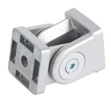
FATH pivot joint, silver, 178-degree adjustable, 2 holes, die-cast zinc, slot size 8. For use with all 40mm and 80mm profile T-slotted rails. Manufacturer part number: 093G40AN.
