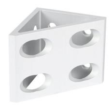
FATH gusseted inside corner bracket, silver, 90-degree, 8 holes, anodized aluminum, slot size 8. For use with all 40mm and 80mm profile T-slotted rails. Manufacturer part number: 093W8806N08.
