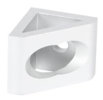
FATH gusseted inside corner bracket, silver, 90-degree, 2 holes, anodized aluminum, slot size 8. Package of 10. For use with all 40mm and 80mm profile T-slotted rails. Manufacturer part number: 093W8404N08.
