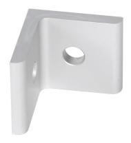
FATH inside corner bracket, silver, 90-degree, 2 holes, anodized aluminum, slot size 8. For use with all 40mm and 80mm profile T-slotted rails. Manufacturer part number: 093WD40.
