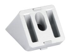
FATH angle connector, silver, 45-degree, 40 x 40mm, die-cast aluminum, slot size 8. For use with all 40mm and 80mm profile T-slotted rails. Manufacturer part number: 093WS40145N08.
