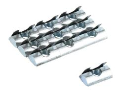
FATH roll-in nut, silver, M8-1.25, zinc plated steel, slot size 8. Package of 10. For use with all 40mm and 80mm profile T-slotted rails. Manufacturer part number: 096028F.
