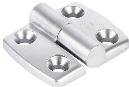
FATH right-hand detachable combination hinge, silver, die-cast aluminum, slot size 8. For use with all 30mm and 60mm profile T-slotted rails. Manufacturer part number: 095A3030RS20.
