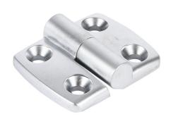
FATH right-hand detachable combination hinge, silver, die-cast aluminum, slot size 8. For use with all 30mm and 60mm profile T-slotted rails. Manufacturer part number: 095A3030RS20.
