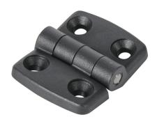
FATH non-detachable combination hinge, black, fiberglass reinforced plastic, slot size 8. For use with all 30mm and 60mm profile T-slotted rails. Manufacturer part number: 095K3030F08.
