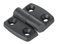
FATH right-hand detachable combination hinge, black, fiberglass reinforced plastic, slot size 8. For use with all 30mm and 60mm profile T-slotted rails. Manufacturer part number: 095K3030R08.
