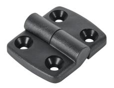
FATH left-hand detachable combination hinge, black, fiberglass reinforced plastic, slot size 8. For use with all 30mm and 60mm profile T-slotted rails. Manufacturer part number: 095K3030L08.
