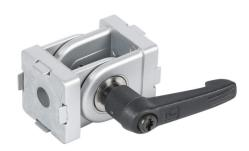
FATH pivot joint with locking handle, silver, 178-degree adjustable, 2 holes, die-cast zinc, slot size 8. For use with all 30mm and 60mm profile T-slotted rails. Manufacturer part number: 093GF30AN08.
